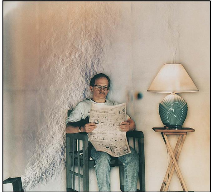
**Figure 4: Full-scale schlieren photograph of a domestic room with person, lamp, and electric space heater.**
