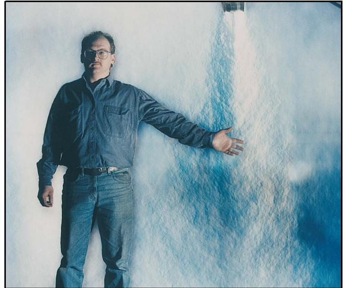
**Figure 6: Full-scale schlieren photograph of an air curtain which produces a planar turbulent jet of heated air.**
