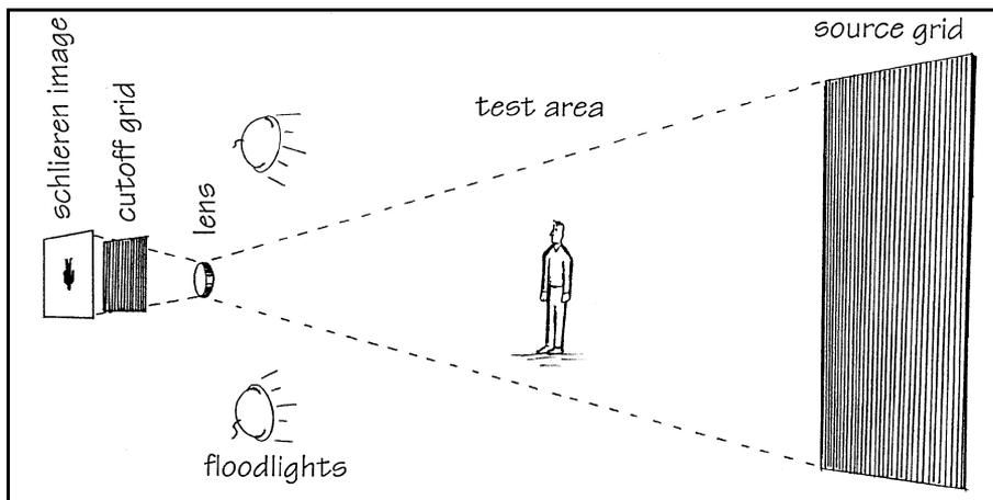
Figure 2: Diagram of full-scale schlieren optical system.
